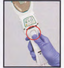
6 Close latch on back of Handpiece.
